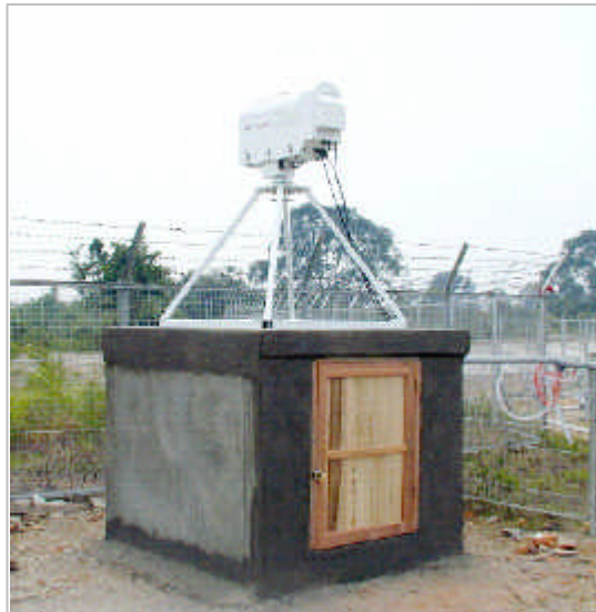
Fig.5. Antenna and RF unit of water vapor radiometer, and major parameters.
