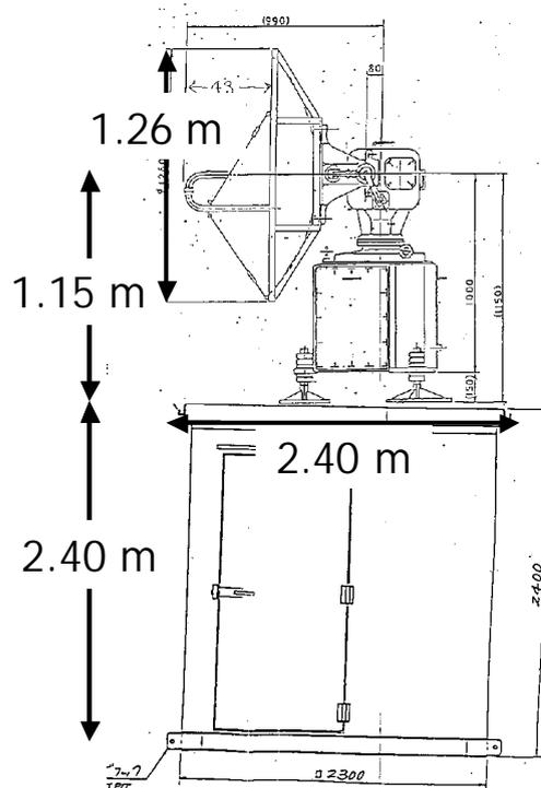
A container (2.4-m height) and a concrete base (1.6-m height) will be used to obtain 7.6 m height at the center of the antenna.
